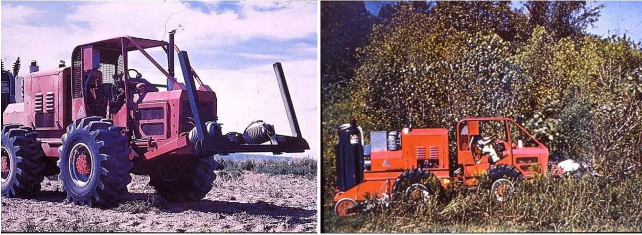
Figure 5. Large self-propelled weeder for scrub control. Note driver is wearing a Faraday suit. Photos Lasco via Dr Mike Diprose.
