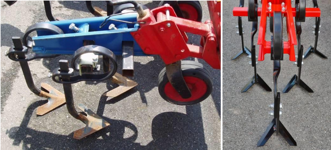
Figure 31. A blade hoes / ducksfeet arranged in staggered pattern. Right photo Horsch.com.
