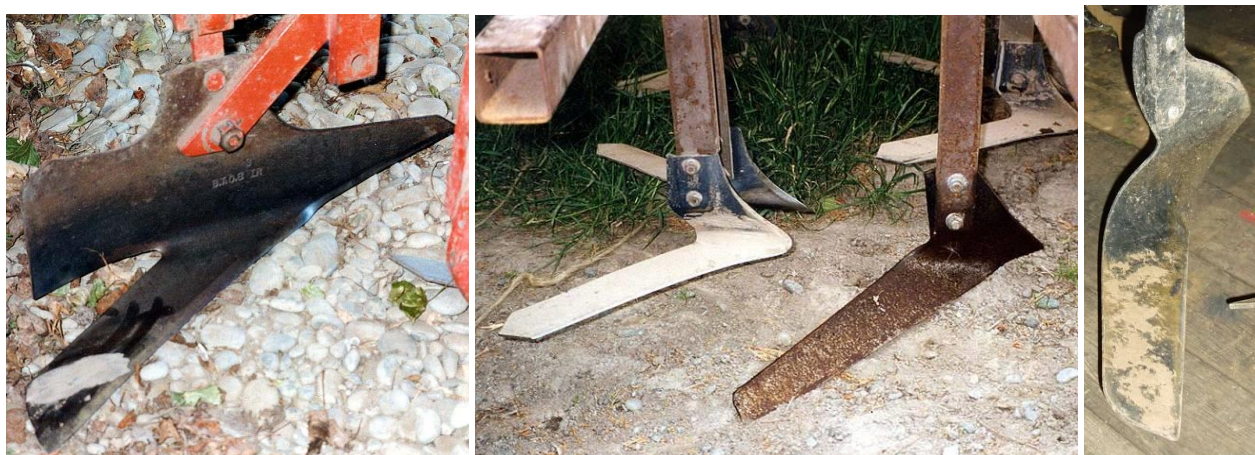
Figure 27. L blade hoes with contrasting front points, heals and shank sizes. Left traditional Nicholson - Webb hoe, middle two generic hoes, right high speed hoe.
