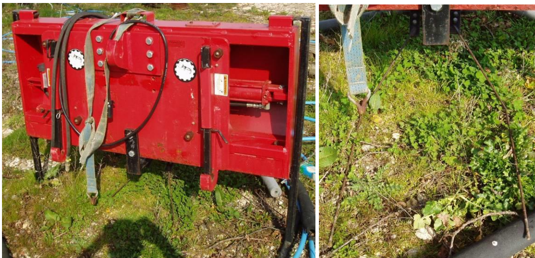
Figure 48. Automated guidance system using crop sensing wands.
