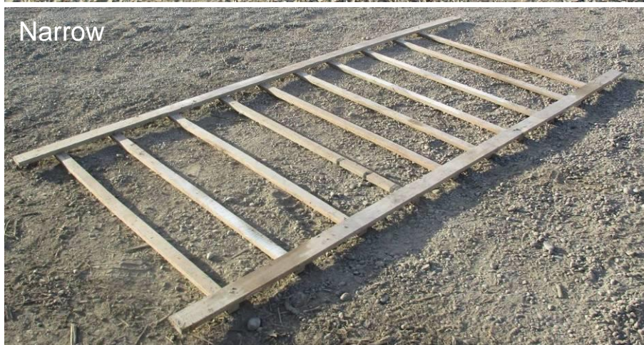
Figure 47. Wooden jigs for setting up a three meter wide row hoe, on 30 cm / 12" wide interrows (crop rows), with wide, medium and narrow intrarow spacings.
