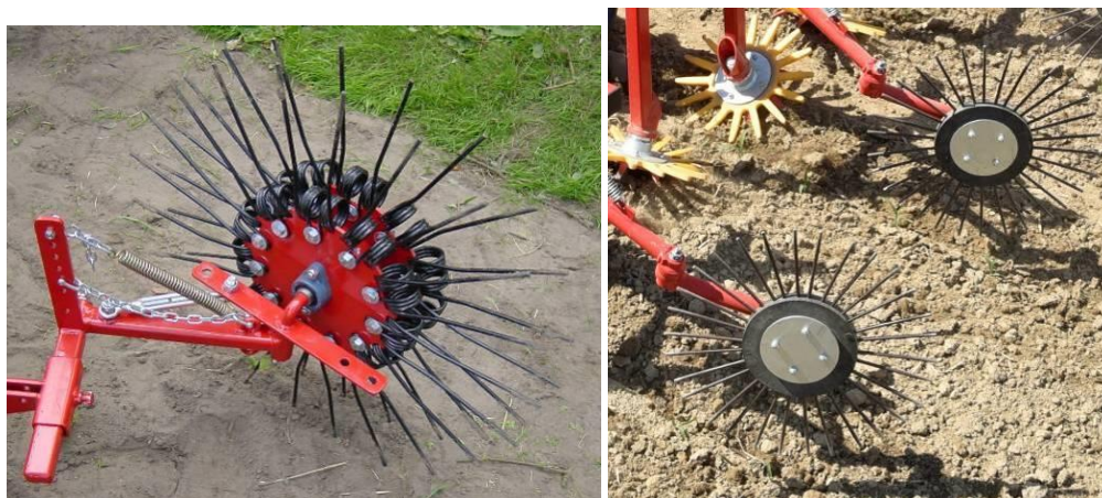
Figure 44. Rotary vertical spring tine intrarow weeders. Left photo Steketee, right photo Einböck.
