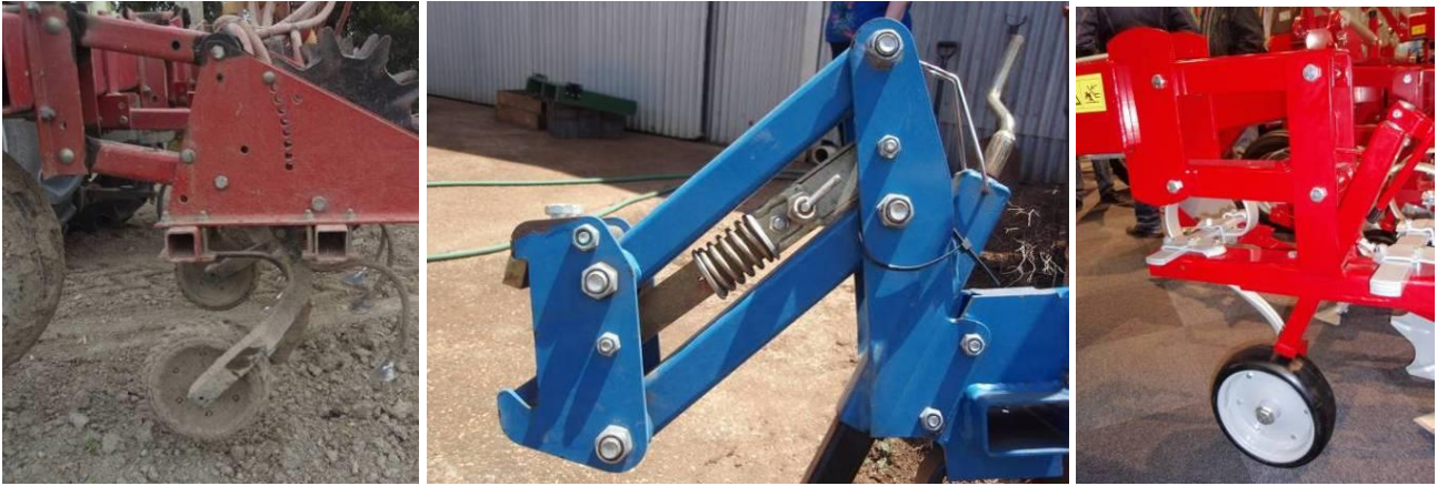
Figure 10. Different parallelogram designs - variations on a theme.
