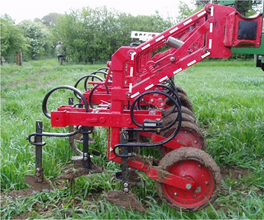
Figure 4. Modular parallelogram weeding unit on a row hoe. Dotted white line highlights the geometric parallelogram shape of the depth control system.
