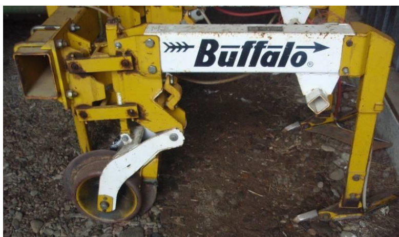
Figure 36. High residue row hoe, with depth wheel incorporating a cutting disk which is followed by a single large A blade hoe.
