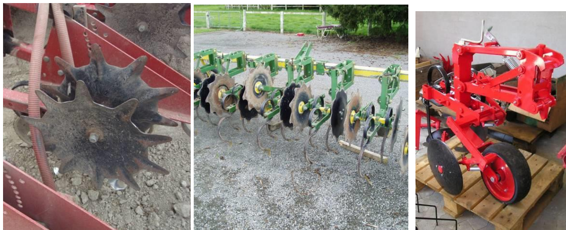
Figure 45. Disk crop protectors. Left and center rolling / walking disks and right concave cutting disks.
