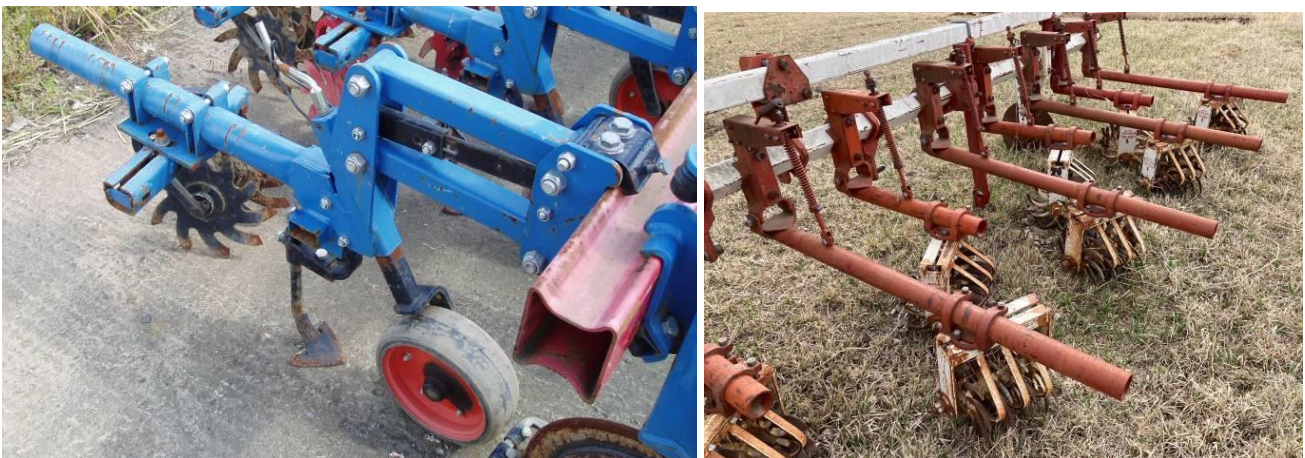
Figure 33. Parallelogram (left) and swinging arm (right) mounting of rolling spider hoes. Right photo Bigiron.com.
