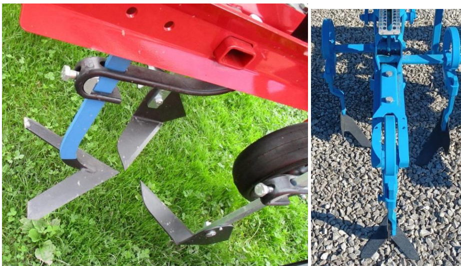
Figure 30. Classic arrangement of L blade hoes next to the intrarow / crop row and an A blade hoe in the center of the interrow.
