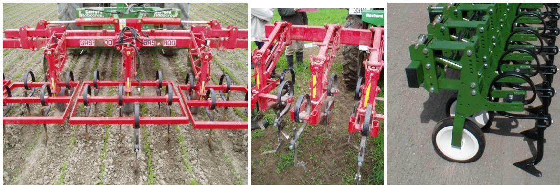
Figure 20. Wide, medium and narrow weeding frames and weeder unit spacings. Right photo Garford Farm Machinery Ltd. garford.com
