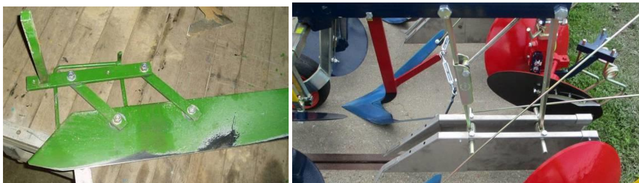
Figure 46. Floating shield type crop protectors, with upswept leading edges to gather and fold crop foliage between pairs of shields.
