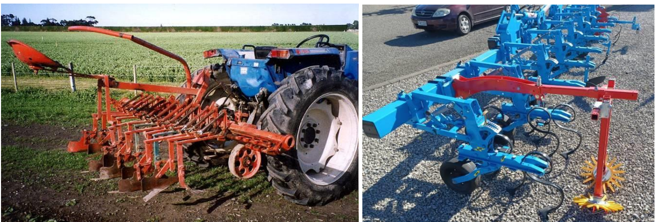
Figure 2. A 1950s Nicholson or Webb interrow hoe (left), modern modular row hoe (right) with multiple parallelogram weeder units and red and yellow finger weeder for weeding the intrarow.
