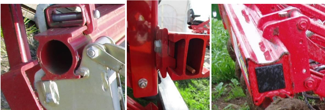
Figure 8. A range of different one sided toolbar clamping systems for weeding units, depth wheels etc.
