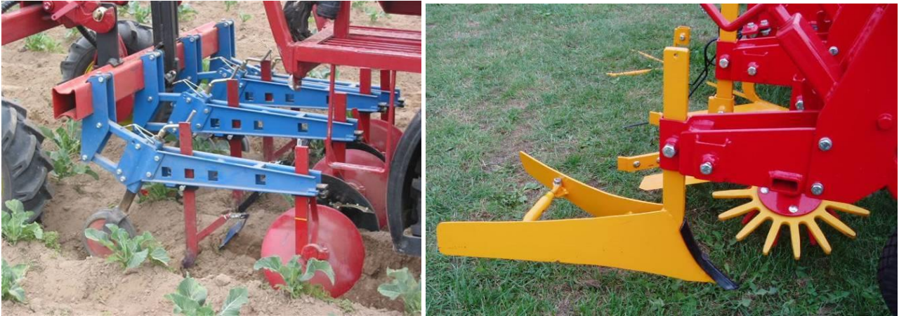
Figure 42. Small concave disks being used for ridging (left) fixed ridger (right).
