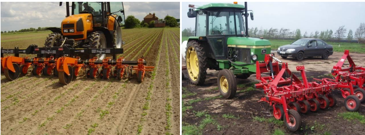
Figure 51. Front mounted interrow hoes. On front three point linkage (left), on dedicated mount (right).
