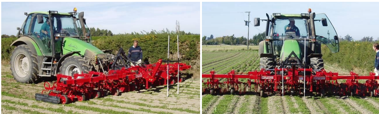
Figure 53. Crop guides on front mounted row hoe.
