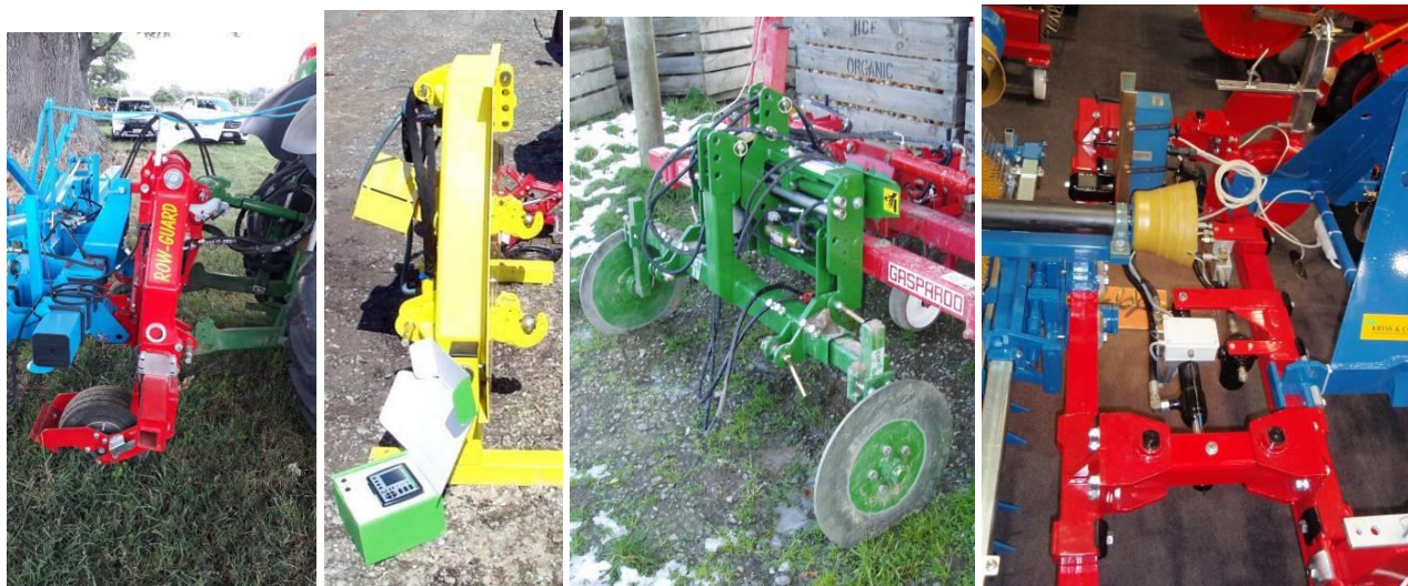
Figure 49. Computer guidance steering systems. Left, three photos hydraulic side shift. Right, parallelogram side shift.
