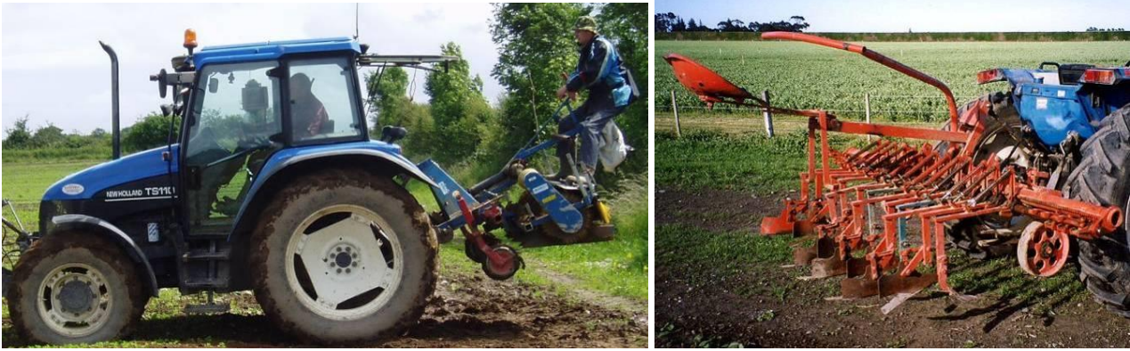
Figure 50. Rear mounted interrow hoes with manual steering system and second operator.
