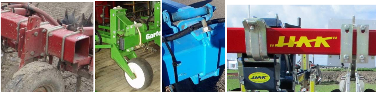
Figure 7. A range of different wrap around attachment systems for weeding units, depth wheels etc.
