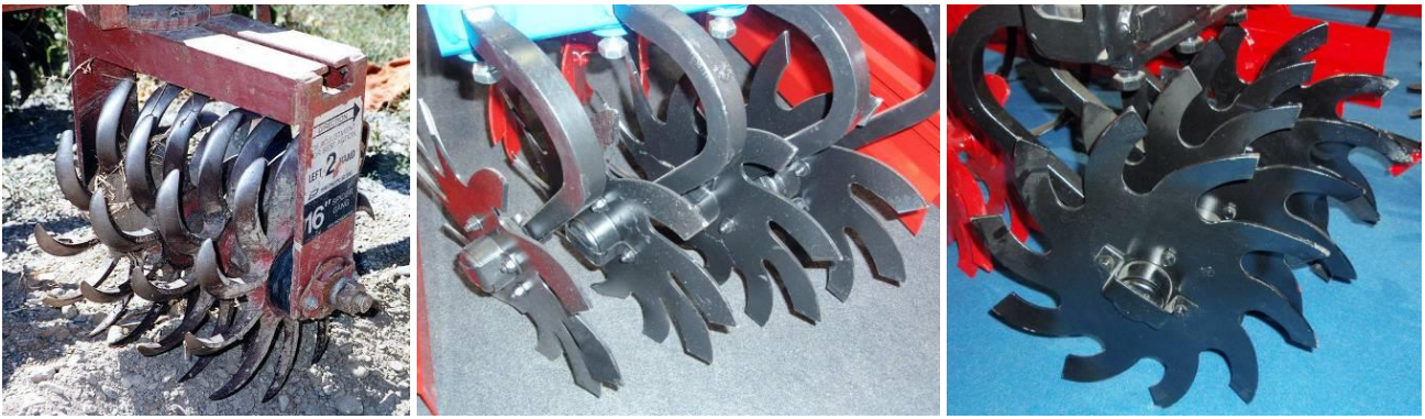
Figure 32. Original Lilliston rolling cultivator (left), rolling spiders / star hoes (center, right).
