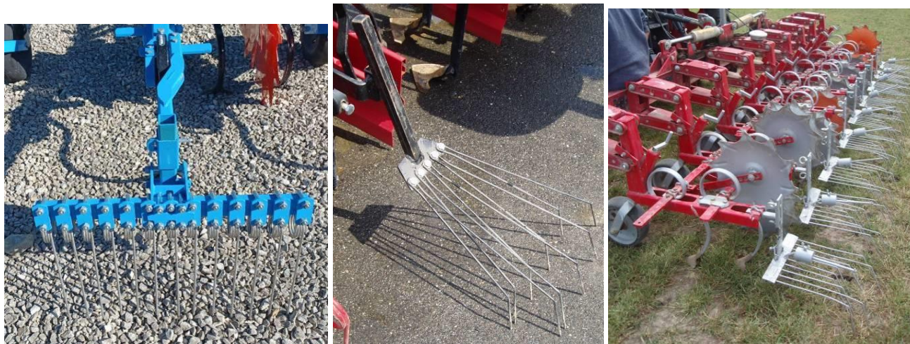
Figure 34. Mini spring tine weeders that improve weed kill by loosening soil, knocking soil off weed roots and further breaking and burying weeds.
