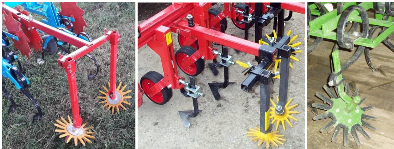
Figure 40. Finger weeder, mounting systems: left and center images, spring tensioned, swing arm, mounting systems; right image, weeding frame mounting on an e-spring clamp.
