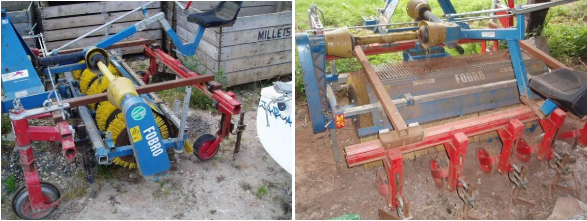
Figure 56. Customisation of a brush weeder with a second toolbar under the hoe drivers feet onto which mini-ridgers have been mounted on telescopes.
