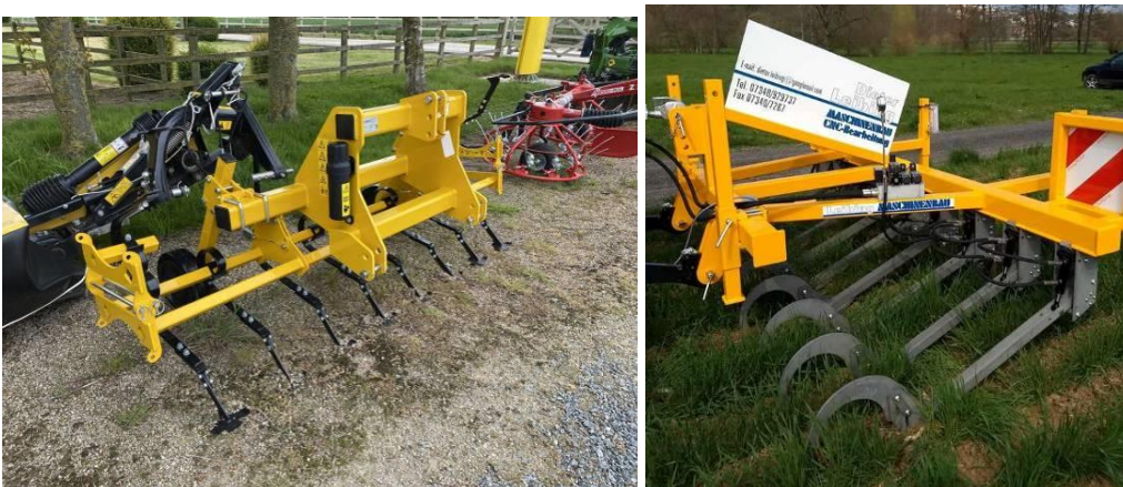
Figure 59. Simple / non-parallelogram interrow hoes for cereal crops. Left photo Claydon Terrablade claydondrill.com. right photo Sickle Hoe Leibing Maschinenbau dieter-leibing.de.
