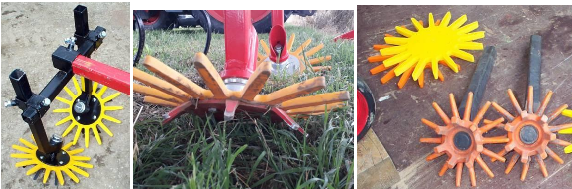
Figure 39. Sandwich design and injection moulded finger weeders.
