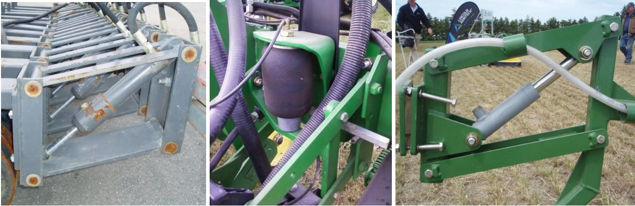
Figure 14. Hydraulic and pneumatic downforce systems on parallelograms.
