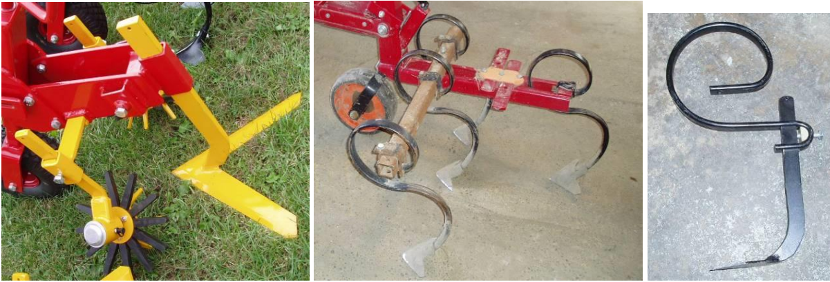
Figure 37. The three main weeding tool legs / springs. Left, fully rigid leg, middle, S spring tine, right e-spring with rigid leg.
