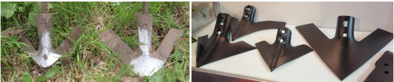
Figure 24. Ducksfoot / goose foot weeder blades which can also be tillage (cultivator) points.
