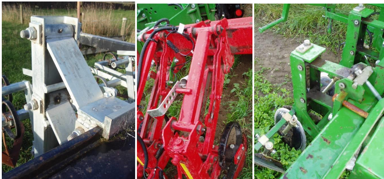
Figure 11. Parallelograms with high horizontal rigidity due to large diameter hinges or bearings that can be greased and parallelogram arms / bars that have zero sideways flex.
