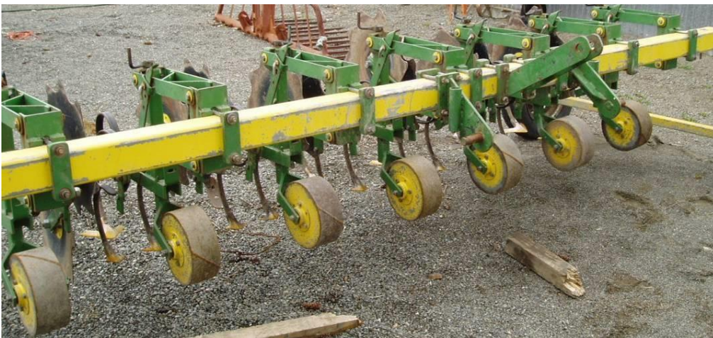
Figure 6. Individual modular parallelogram units (green) attached to toolbar (yellow).
