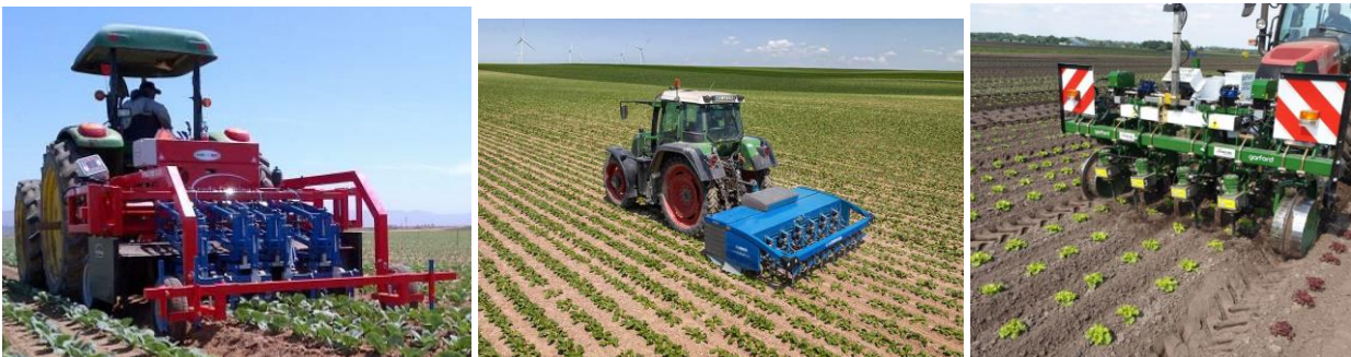
Figure 38. A range of discriminatory intrarow weeders (which include interrow weeding tools). Left photo FerrariGrowtech.com Remoweed, center photo Lemken.com IC-Weeder AI, right photo Garford.com Robocrop in-crop weeder.
