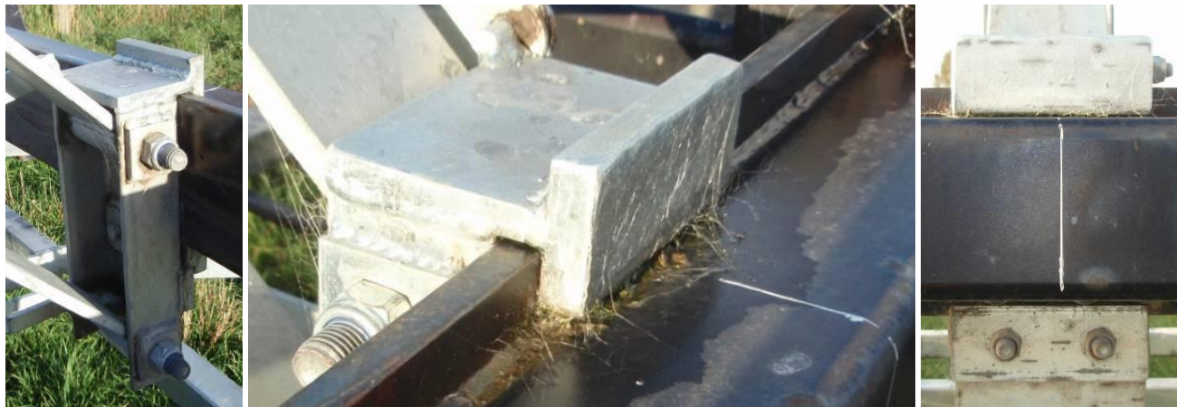
Figure 9. One sided toolbar with drop-in-place mounting system.
